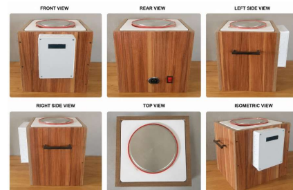
Fig. 4. Constructed prototype of the IoT based solar powered DC cooking plate.
