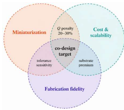
Fig. 3 Interconnected Challenges and Co-Design Trade-offs in Bandpass Filter Design
