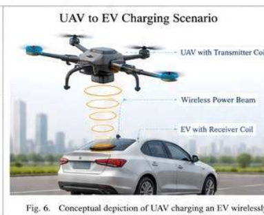
Fig. 6. Conceptual depiction of UAV charging an EV wirelessly.
