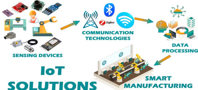
Figure 1. Information Flow within the IoT Paradigm. Data collected by sensing devices installed throughout industrial facilities or used for worker monitoring are transmitted through wired or wireless communication technologies to a centralized data-processing platform. The collected information is then analysed to generate valuable insights related to production quality, equipment condition, operational progress, energy consumption, environmental pollution, and worker well-being.
