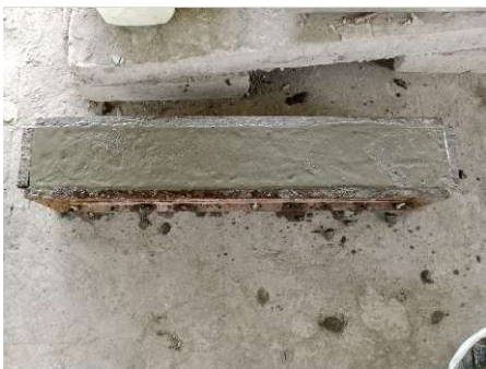
Fig.10 Casting of GFRP reinforced beam
