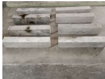
Fig.12 GFRP reinforced beams
