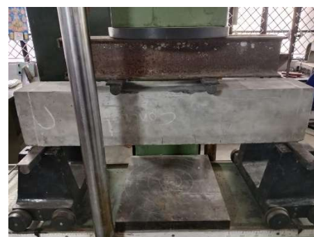
Fig.23 Test setup of control beam subjected to fire
