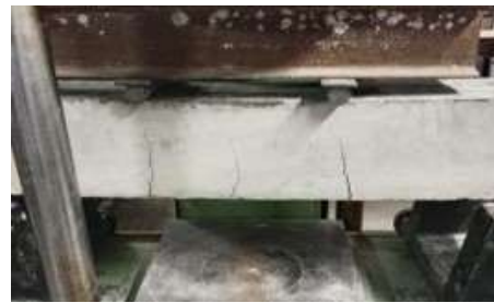
Fig.28 Failure crack pattern of beam with retardant additives (Chitin)
