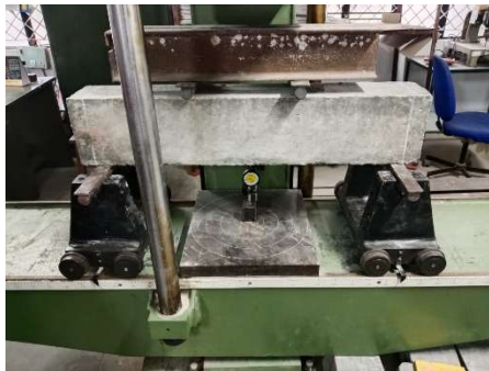
Fig.17 Test setup of beam with retardant additives (Metakaolin)
