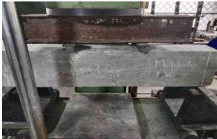
Fig.33 Failure crack pattern of beam with retardant additives (Metakaolin) subjected to fire
