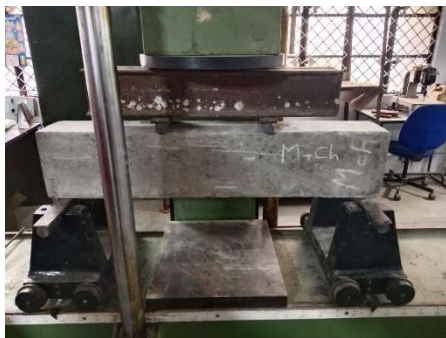
Fig.18 Test setup of beam with retardant additives (Combined Chitin & Metakaolin)
