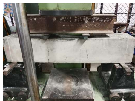
Fig.16 Test setup of beam with retardant additives (Chitin)
