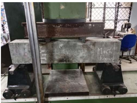
Fig.26 Test setup of beam with retardant additives (Combined Chitin & Metakaolin) subjected to fire
