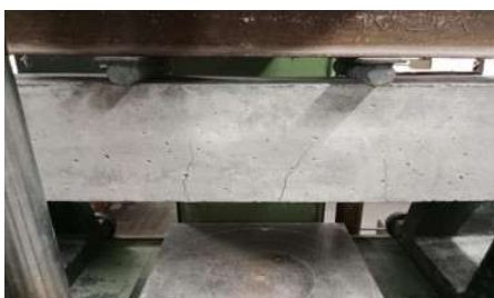
Fig.27 Failure crack pattern of control beam
