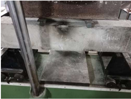
Fig.24 Test setup of beam with retardant additives (Chitin) subjected to fire
