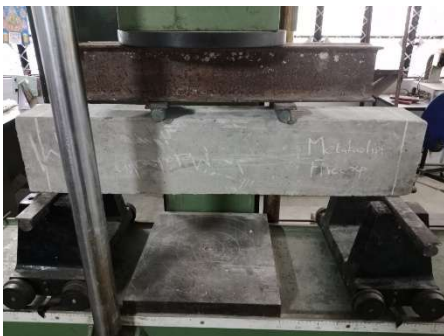
Fig.25 Test setup of beam with retardant additives (Metakaolin) subjected to fire
