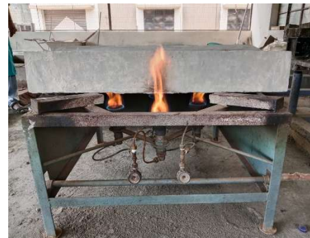
Fig.19 Fire exposure test on GFRP Reinforced Beams
