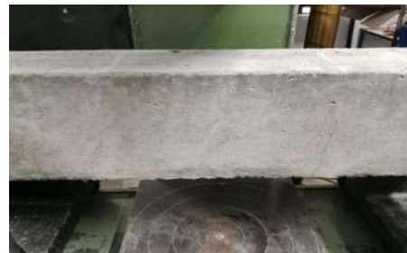
Fig.29 Failure crack pattern of beam with retardant additives (Metakaolin)
