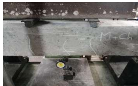
Fig.30 Failure crack pattern of beam with retardant additives (Combined Chitin & Metakaolin)
