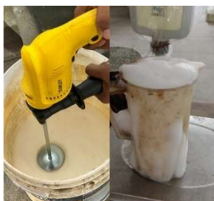
Fig.6 Foam half life test
