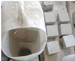
Fig.12 Water absorption test
