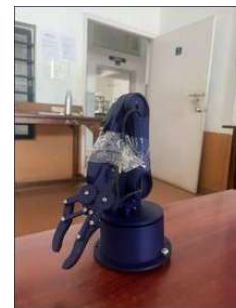
Fig. 8. Custom 3D-Printed Robotic Arm for Assistive Object Manipulation
