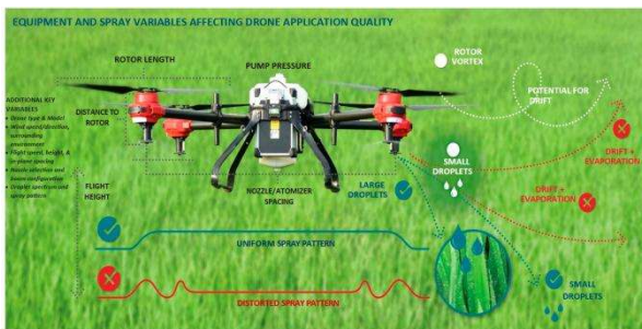
Fig. 3. Working Mechanism of Drone Spraying
