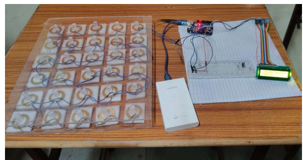
Fig1. Experiment setup of the piezoelectric tile
