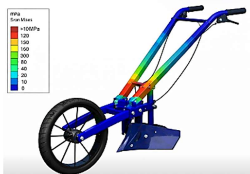
Fig.5. Stress Distribution Obtained from Simulation
