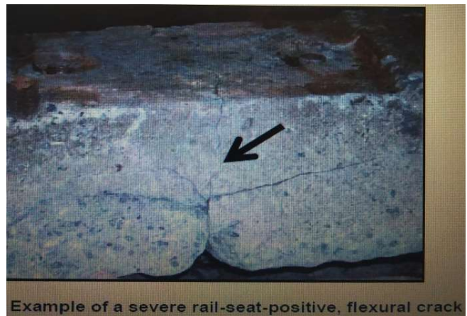
Fig.2 An illustration of a severe, flexural, rail-seat-positive crack
