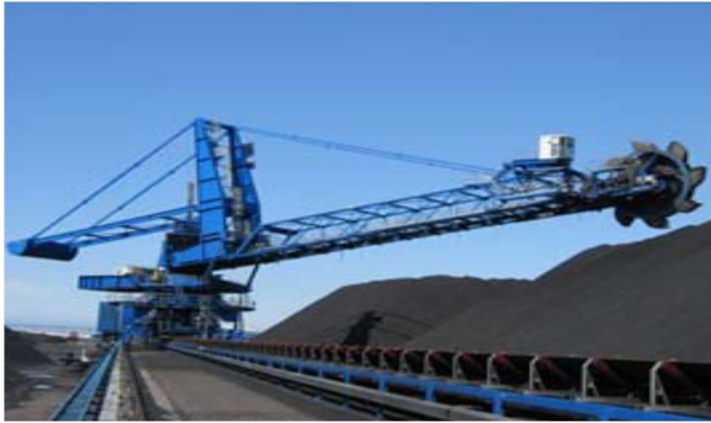
Fig 4: Stacker cum reclaimer in coal yard
