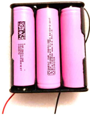
Fig. 6 Lithium-ion Battery Pack
