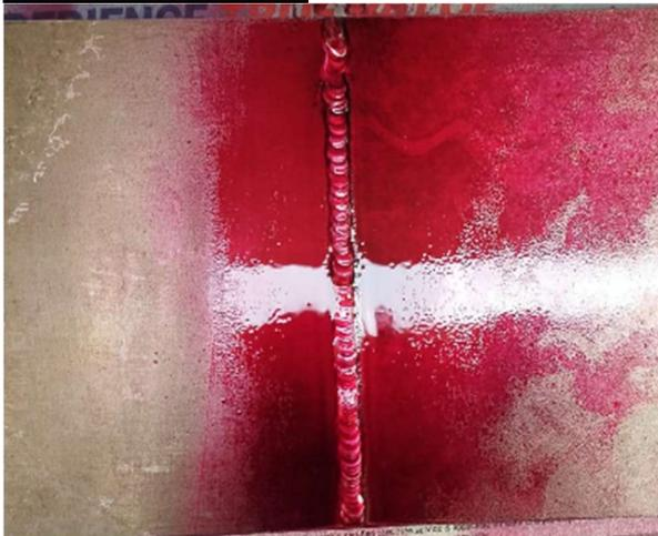
Fig 8: DP Testing after applying penetrant
