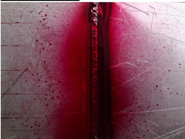
Fig 10: DP Testing after applying penetrant
