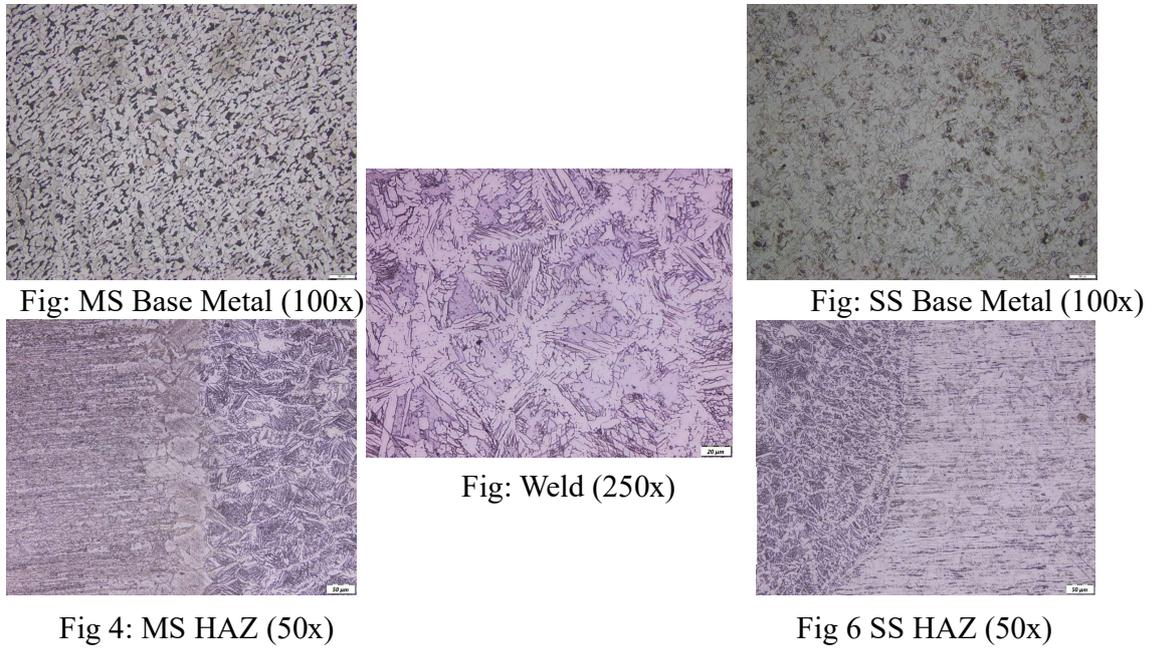
**Figure 4** – Optical microstructure of LBW joint
