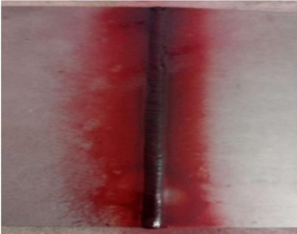
Fig 6: DP Testing after applying penetrant
