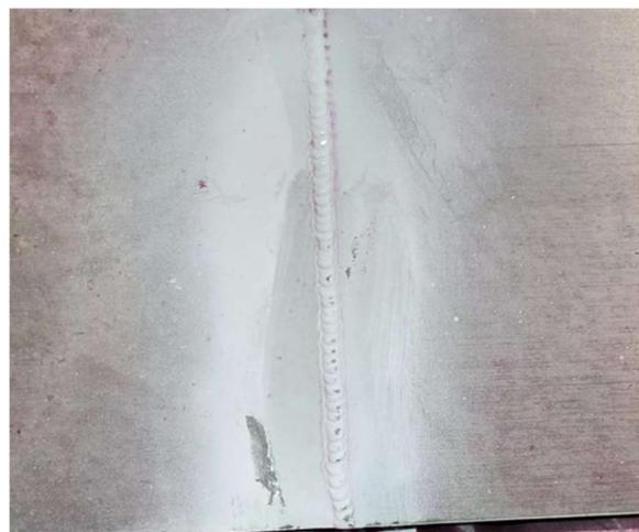
Fig 9: DP Testing after applying developer
