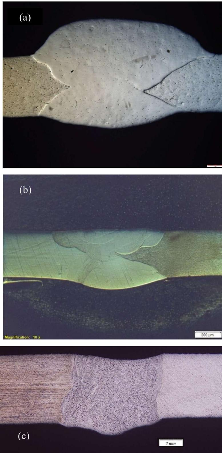
**Figure 2** – Macroscopic appearance of dissimilar joints: (a) GTAW, (b) FSW, (c) LBW
