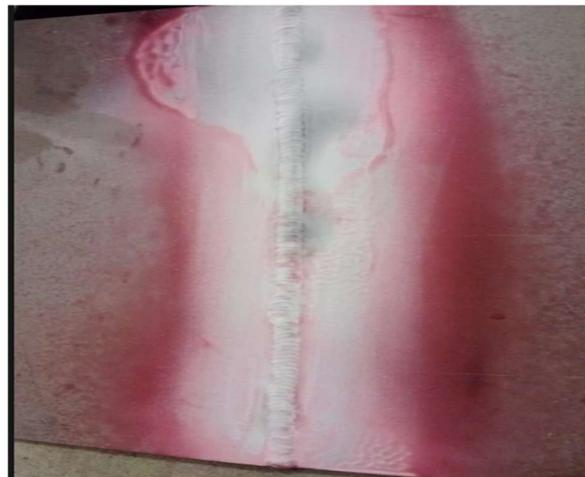
Fig 7: DP Testing after applying developer
