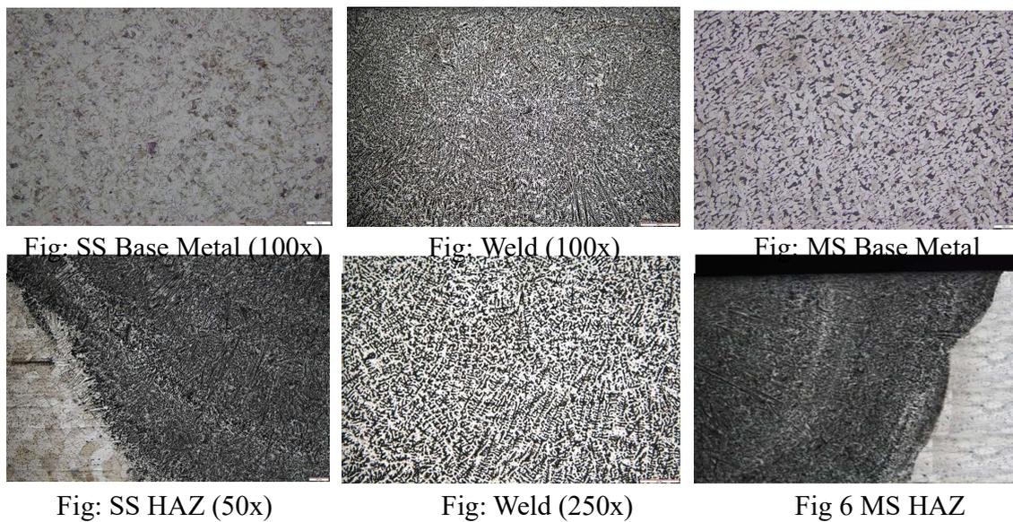
**Figure 5** – Optical microstructure of FSW joint
