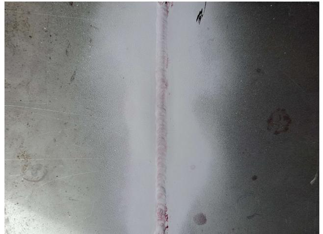
Fig 11: DP Testing after applying developer
