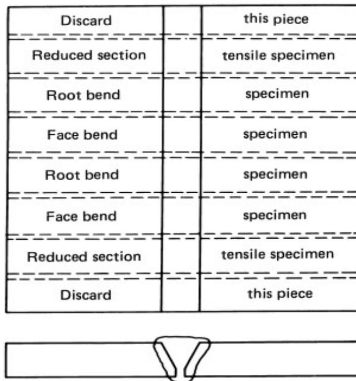
Fig 1: Weld Test Coupon Extraction Plan
