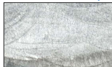
(Fig. 3: Stereo microscope image showing lack of fusion defect at interlayer interface.)
