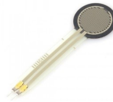
Fig. 1. Force Sensing Resistor (FSR) sensor used in the project.
