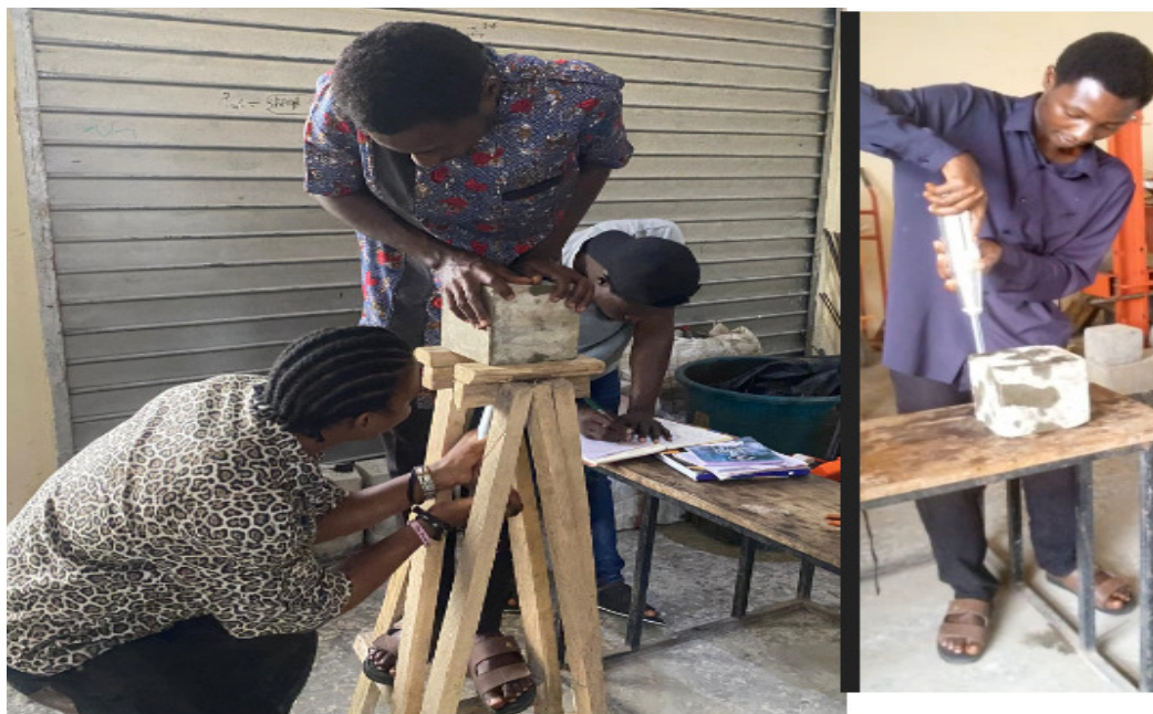
Figure II: Testing of concrete samples with varying direction
