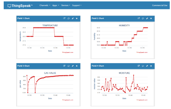
Fig. 7. ThingSpeak cloud charts for temperature, humidity, gas values, and moisture levels
