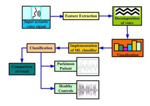
A block diagram is shown below that explains the entire process of the proposed Parkinson's disease detection system using voice recordings signals and machine learning approaches. This starts with the acoustic voice signal, where speech signals are extracted from individuals through vowels prolongation or speech signals. These raw voice signals hold significant information about the vocal handicaps created by Parkinson's disease.
