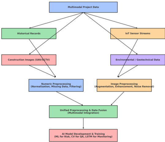
Figure 1. Multimodal Data Processing Pipeline for AI-Based Risk and Quality Monitoring
