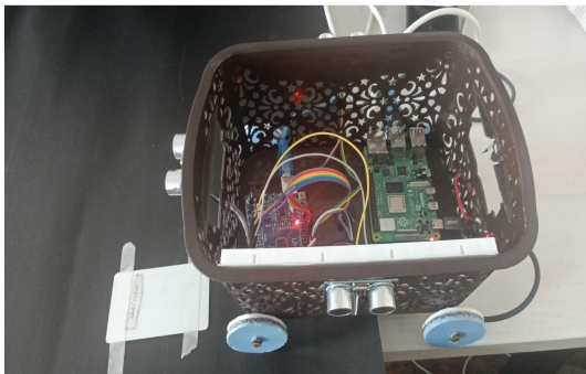
Fig.4: Hardware setup of the IoT-Based Smart Trolley showing integration of Raspberry Pi 3, ultrasonic sensors, RFID module, and speaker–microphone interface.
