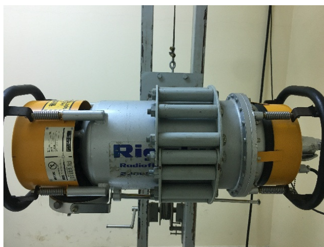
Fig. 1. Rigaku-200EGM X-ray generator: a) controller, b) X-ray tube
