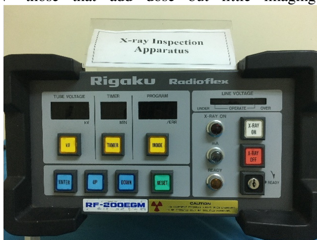
Fig. 1. Rigaku-200EGM X-ray generator: a) controller, b) X-ray tube
