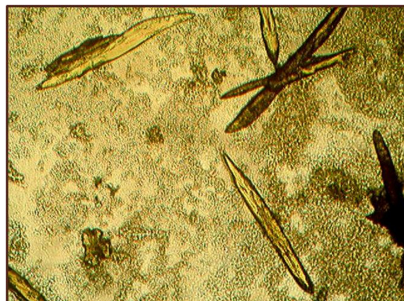
Figure Fiber Stained with Phloroglucinol +conc.HCL (1:1)
