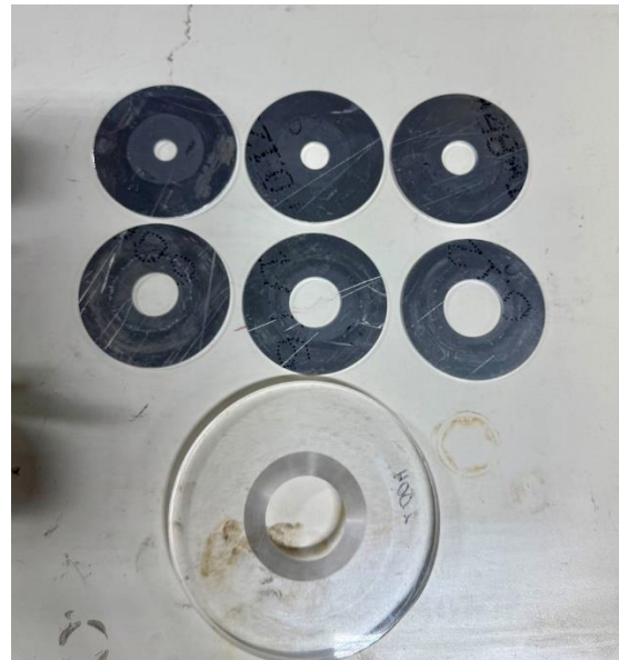
Figure 3. 2-inch orifice plate's arranged as follow: the top row (left to right) contains beta ratios of 0.3, 0.4, and 0.5; the second row (left to right) contains beta ratios of 0.6, 0.7, and 0.8. The 4-inch orifice plate is positioned at the bottom.
