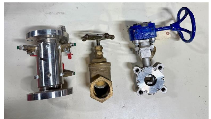
Figure 4. Tested components, including the Venturi meter (left), gate valve (middle), and the butterfly valve (right).
