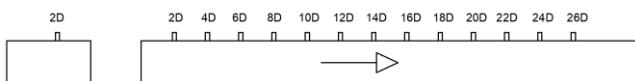
Figure 2. Schematic of the experimental test section showing pressure tap locations at 2D intervals downstream (from 2D to 26D). The upstream tap is located at 2D upstream of the test section.
