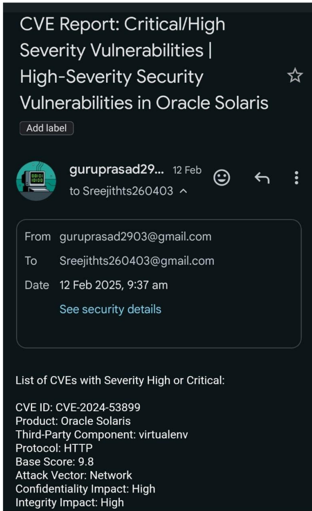
Fig.1.10: Screenshot of a security advisory email reporting CVE-2024-53899 in Oracle Solaris, with a CVSS score of 9.8. The vulnerability impacts the virtual env component and is exploitable via network using the HTTP protocol.
