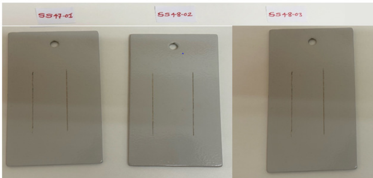
Fig. 1: Digital photographs of scribed SS painted sample exposure up to 24 hours in salt spray chamber.
