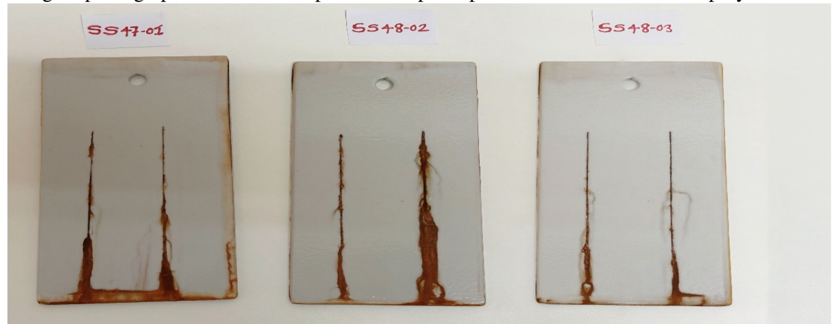
Fig. 04: Digital photographs of scribed SS painted sample exposure to 750 hours in salt spray chamber.
