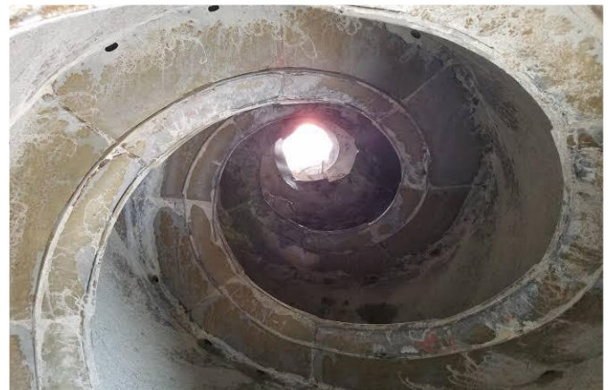
Figure 4. blade covers with wear-resistant materials
