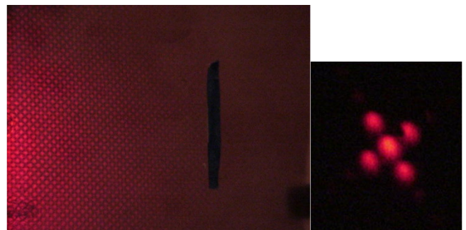
Photograph 7. Image of the object in the observation plane with a filter that allows only the central dot to pass.
