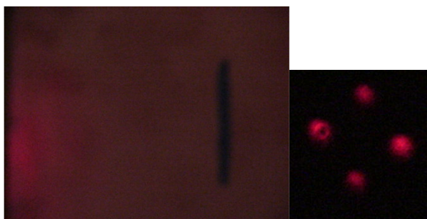
Photograph 10. Image of the object in the observation plane with a filter that allows only order 2 to pass.
