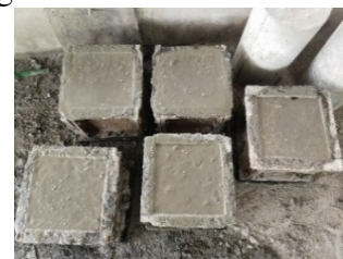
FIG 3 CASTING OF CUBES
