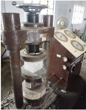
FIG 4 COMPRESSIVE TEST OF CUBES
