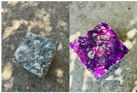
Fig.14 Carbonation Depth test in CBA concrete
