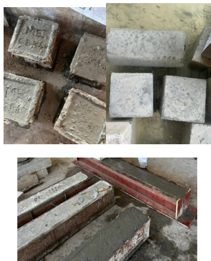
Fig 5 Casting and curing of Specimen
