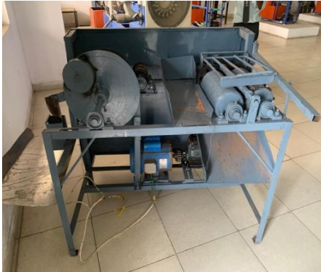
Fig No: 4 Fabricated Coconut dehusking Machine
