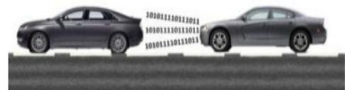
Fig1.1 First Scenario of Vehicle to Vehicle Communication Using VLC
