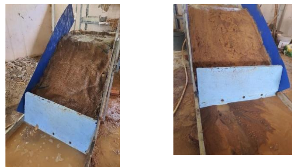
Fig 8: Slope with both jute and retaining wall before and after 150mm/hr of artificial rainfall
