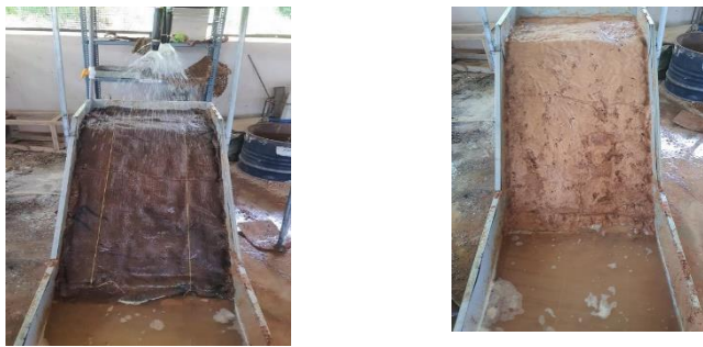
Fig 6 - Slope with jute fibre before and after 150mm/hr of artificial rainfall
