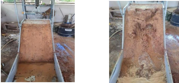
Fig 5: Normal slope before and after 150mm/hr of artificial rainfall
