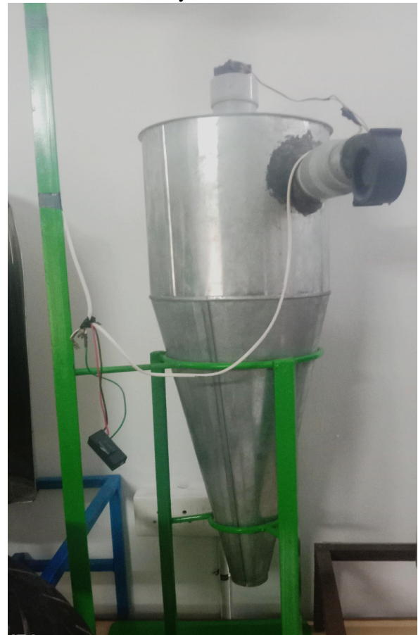
Fig.1. Solar Powered & Centrifugal Air Filtration Machine Setup
