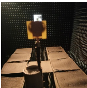
Fig. 10.11 Anechoic Chamber for proposed patch antenna.
