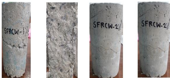
Figure 10: Shows development of cracks in the cylindrical specimens of SFRCW under splitting-tensile load
