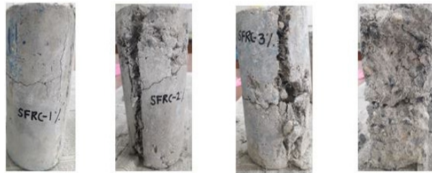
Figure 9: Shows development of cracks in the cylindrical specimens of SFRC under splitting-tensile load
