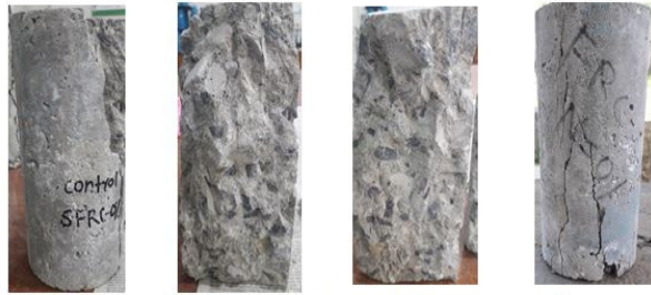
Figure 9: Shows development of cracks in the cylindrical specimens of SFRC under splitting-tensile load
