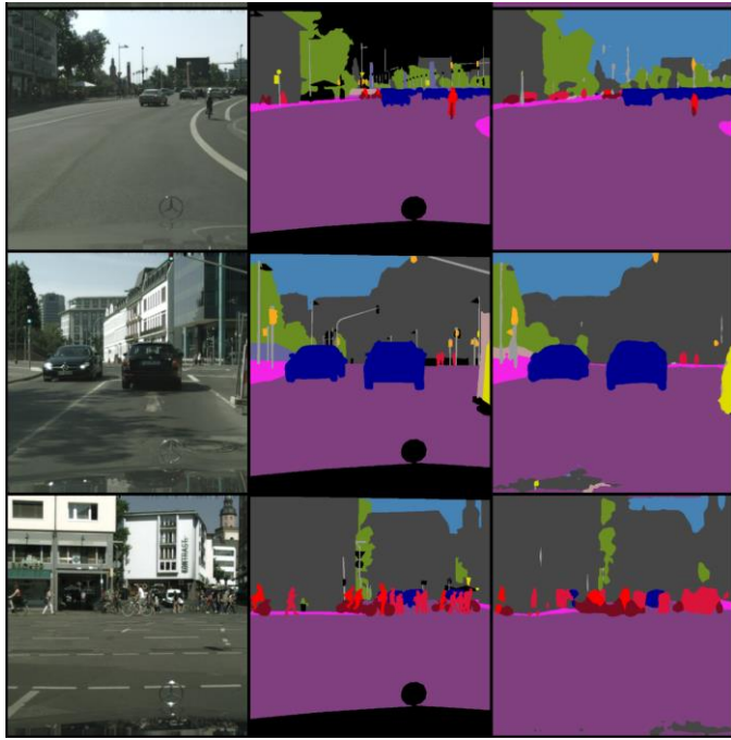
Fig 9: Real image frame (left) vs Ground Truth (middle) vs Predicted Segmentation (right).
