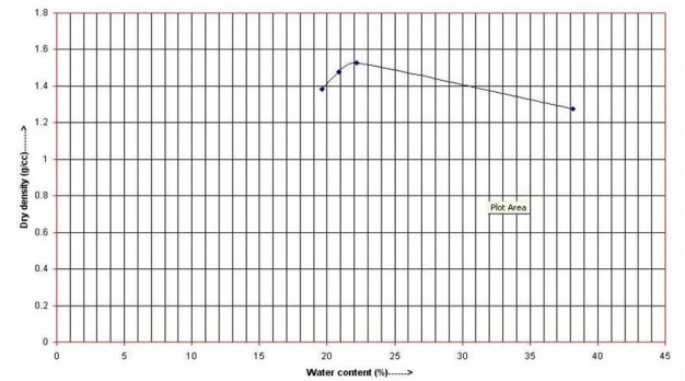
Fig-4: Proctor compaction Test with swelling soil+20% GNA
