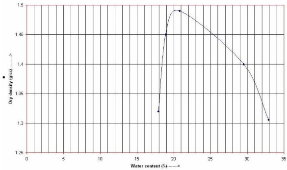
Fig-2: Proctor compaction Test for expansive soil
