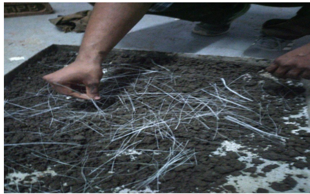
Figure 2 : mixing sisal fibers in soil
