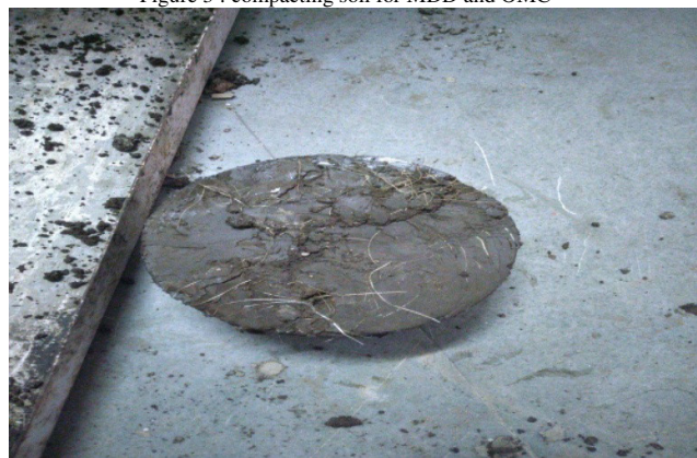
Figure 4 : sisal nailed soil sample
