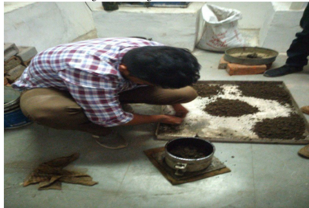
Figure 3 : compacting soil for MDD and OMC
