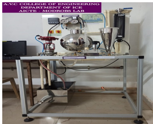
Figure 1- Labeled Photograph of the Conical & Spherical Tank Level Process Trainer
