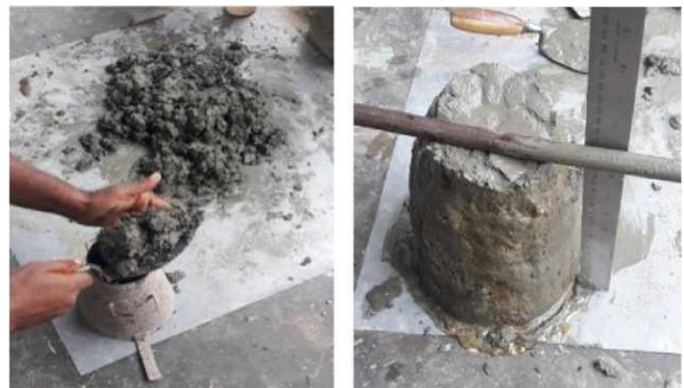
Fig. 2. Slump test (a) mould preparation (b) slump value measurements
