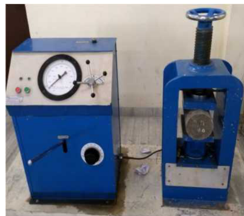
Fig.4 SPLIT TENSILE STRENGTH TEST IN CTM
