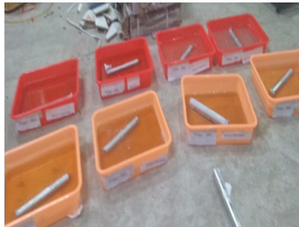
Fig.1 Specimens Quenched in media
