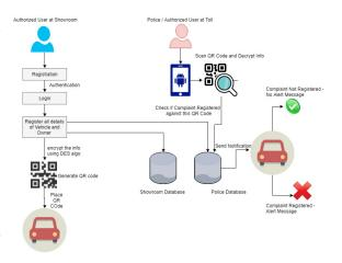
A description of the program architecture is presented. Subsystem design or Block diagram, Package Diagram, Deployment diagram with description is to be presented.
