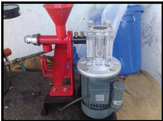
Fig.1: Motorized operated oil expeller used for expelling oil from vegetable seeds [26]
