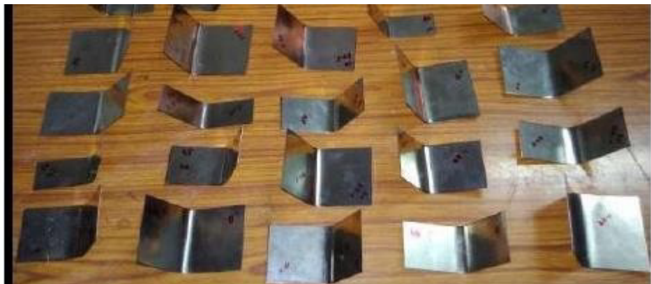
Figure 4.2: AISI 304 material after bending
