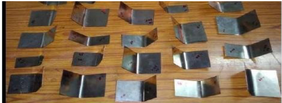
Figure 4.2: AISI 304 material after bending
