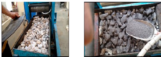
Figure 1: Compaction and rutting using RCRA
