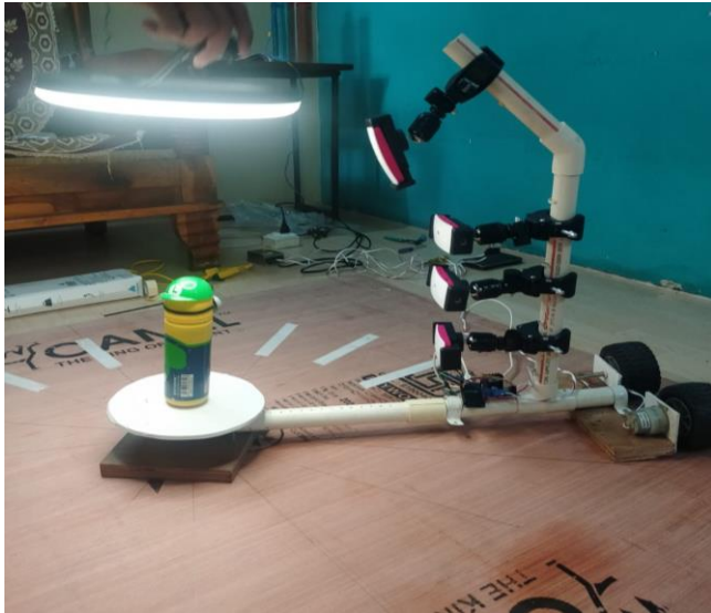
Fig 1 Mechanical arrangement of cameras and lights
