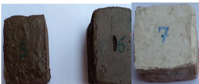
Fig. 2: Unstructured (Sample 1) and Prestructured (Sample 2) And Elastomer with Steel net (Sample 3)
