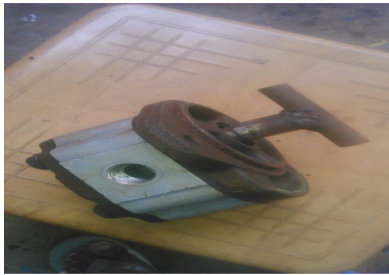
Fig.4. photograph of Oil rotor Pump
