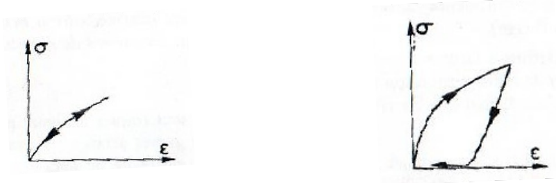
Figure 1- Linear elastic flow Figure 2 -Viscoelastic flow
