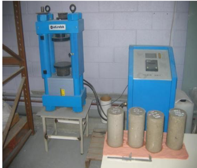
Figure 9- SNCC compression testing machine
