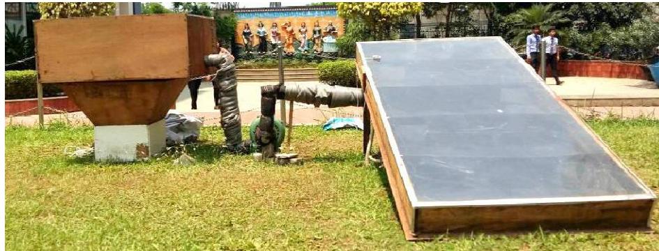
Fig.4 Complete experimental setup of the indirect solar dryer [24]
